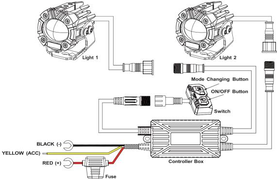
2. Install the lights: Determine the mounting locations to install the lights, harness, and switch. Use the provided mounting accessories shown below to securely mount the lights. Using zip ties, secure any loose wiring.
