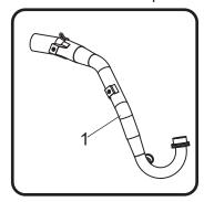
2. Install (No. 4) *HT SHLDR77*, muffler clamp heat insulator onto (No. 3) *12130-MPCX*, muffler clamp and trim excess heat insulator.
