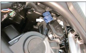
12 Plug the PC6 wiring harness in-line of the bike's TPS and the stock wiring harness.
