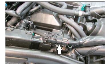
7 Locate and unplug the Fuel Injector sub-harness connector just below the fuel tank on the left side of the bike.
