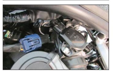
13 From the right hand side of the bike, locate and unplug the stock Crank Position Sensor connectors.
