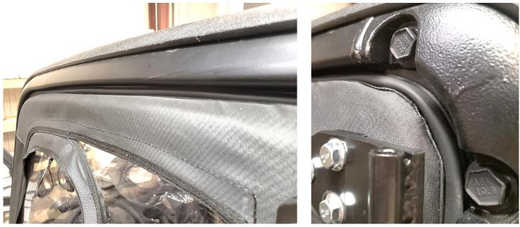
**16.** Adjust the door in and out using the slots in the Upper Door Mount (H) and Lower Door Mount (I). Use these slots to increase or decrease compression on the door gasket. See images above for proper gasket compression
