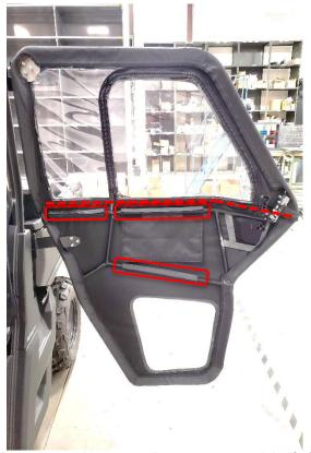
**4.** The upper and lower textiles come on each half of the frame but you will need to attach the halves together and ensure they are properly secured. The highlighted areas are the main areas you will need to address. There are 3 center flaps that wrap around the tubing along with the 2" Velcro seam between the upper and lower textiles.
