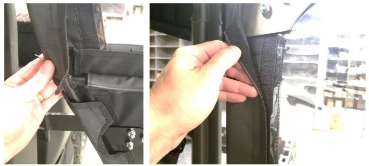
6. Make sure the perimeter flap is centered and secured around the entire frame.
