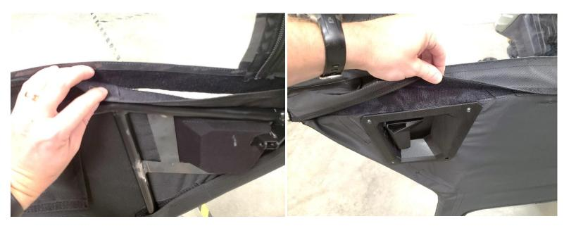
**7.** Pull the lower textile upwards and the upper textile downwards to line up the 2" seam Velcro so that the textile is snug and lines up evenly.
