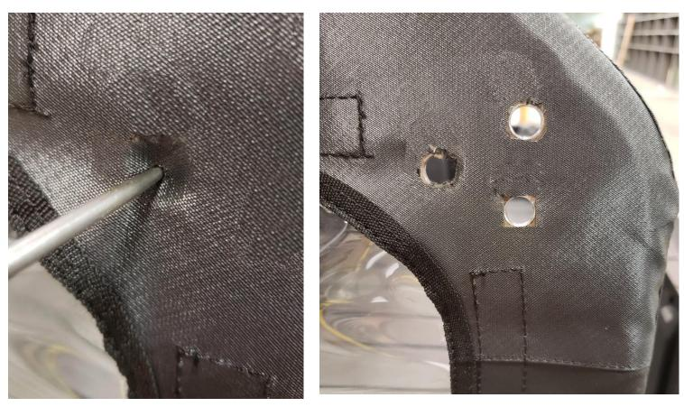
**9.** Holes need to be cut in door textile panels in order to mount the Upper and Lower Sliding Hinges. **Ensure textiles are tight and fit as desired before marking and cutting holes.** Take a sharp scribing tool and punch a small hole through the textile indicating the center of the slot. Take a razor blade and carefully cut out the small amount of textile so that the supplied M8 bolt may pass through the plate and the textile. Repeat this process for the lower mounting location.
