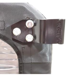
**10**. Pass M8x25mm flange bolts through the Upper Door Hinge Plate (F), textile, then the welded on door plate. Attach using M8 flange bolts and lock nuts as shown. Do not fully tighten at this time. Hinges are slotted for door adjustment.
