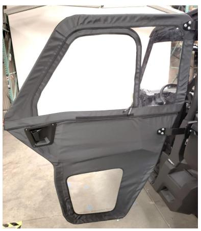
**8.** The textiles should appear taught but not bursting at the seams. If they are too tight in warmer weather, they will only become tighter in cooler temperatures. If you are installing these doors in the summer, give yourself some slack in the textile fit-up so that when winter rolls around, the textiles will fit properly.
