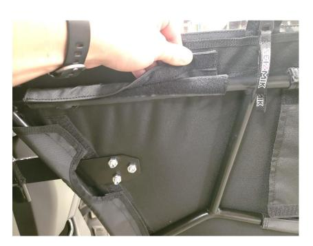
**5.** The flaps wrap all the way around the center frame tubes as shown in the picture above. Secure and wrap these at tightly as possible. Repeat for all center flaps.
