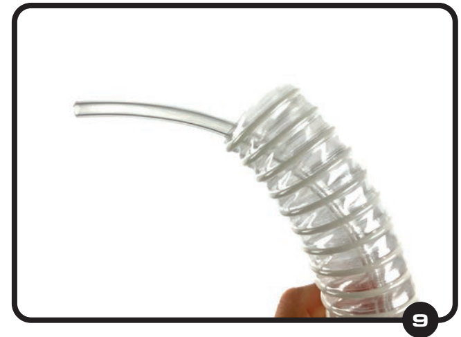
Feed the 6MM Hub Line so that it runs through the entire Hose and exposes itself to the helmet end and has a few inches of extra Hub Line.
