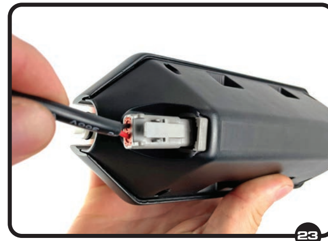
Make sure that when you insert the Gray Deutsch Connector you hear a secure, "Click" to assure that the part is inserted correctly.
