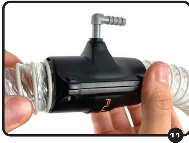
Bring the air hose to the Hub, apply a small amount of silicone onto the threads, and thread the hose onto the Hub in a counter-clockwise direction.
