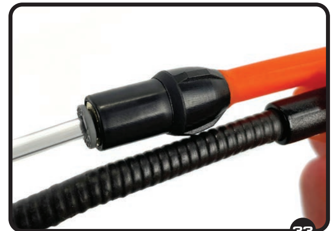
Run the 4mm AquaCom Line into the AquaCom's Grey Legris.
