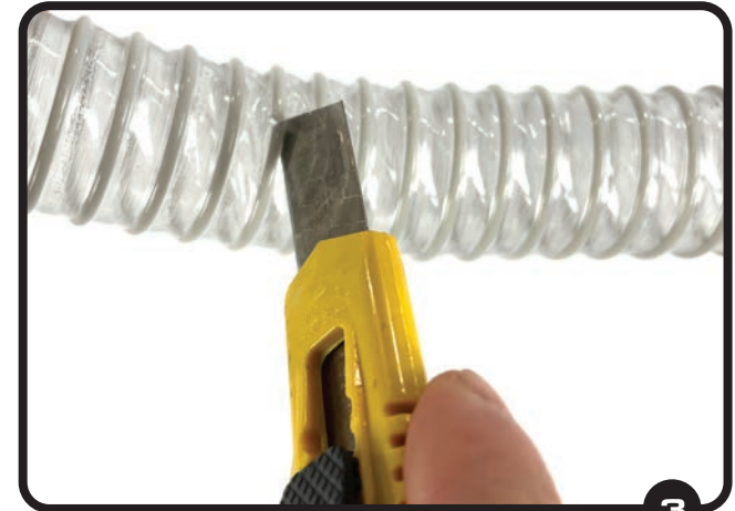
3 Using a sharp knife, pierce the hose making a clean cut in a 360 degree fashion. Expose the wire core and prepare to cut it.
