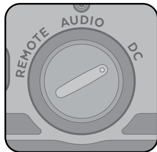
Turn Auto-Turn-On Switch to DC
