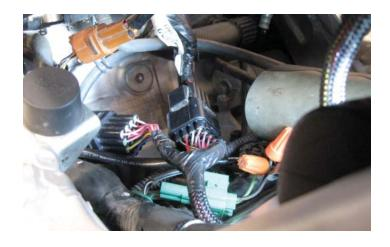
Plug the matching pair of connectors of the PC6 harness in-line of the stock connectors.
