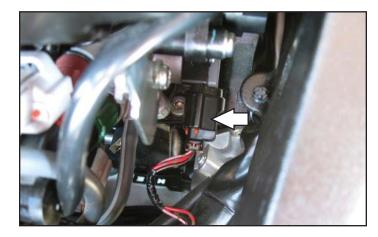
10 Plug the 3-pin connectors from the PC6 in-line of the stock TPS and wiring harness.
