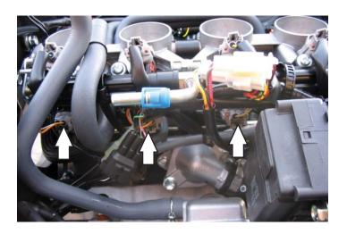
6 Unplug the stock wiring harness from each of the LOWER injectors.
