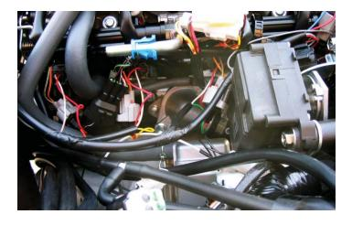
7 Plug the connectors from the PC6 in-line of the stock LOWER injectors and the stock wiring harness.
