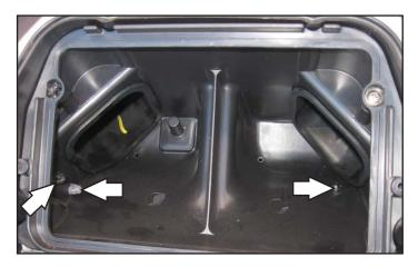
8 Unplug the stock wiring harness from each of the four injectors.
