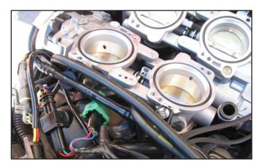
13 Plug the connectors from the PC6 in-line of the fuel injectors and stock wiring harness.
