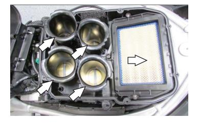
6 Remove the velocity stacks and the air filter.
