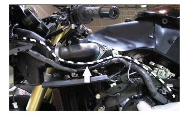
4 Lay the PC6 next to the gauge panel temporarily and route the PC6 harness along the stock wiring harness to the throttle body connection. Use the supplied zip ties to secure the PC6 wiring harness.
