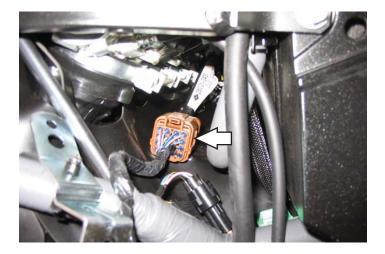
3 Disconnect the stock wiring harness from the throttle body harness.
