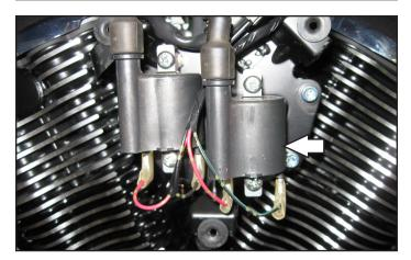
10 Plug the PC6 coil connectors in-line of the stock wiring harness and Ignition coils.
