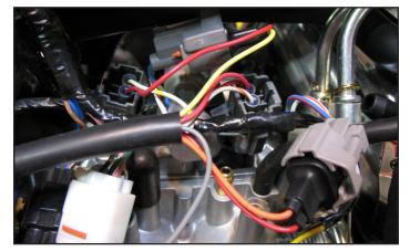
6 Locate the Throttle Position Sensor connector.
