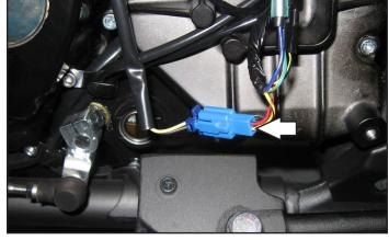
13 Unplug the stock crank sensor connector.
