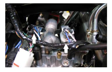
4 Unplug the stock wiring harness from both of the fuel injectors at the top of the throttle bodies.
