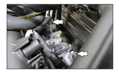
Plug the PC6 wiring harness in-line of the Fuel 8 Injectors and the stock wiring harness.
