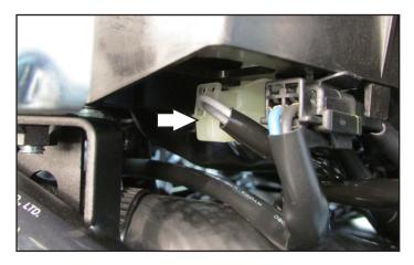
15 Just below the regulator/rectifier, locate and unplug the stock connectors for the bike's Crank Position Sensor.
