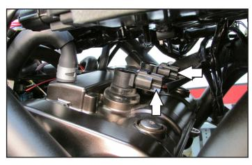
12 Unplug the stock wiring harness from both of the Ignition Coils.
