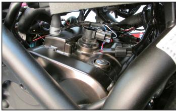
13 Plug the PC6 wiring harness in-line of the Ignition Coils and the stock wiring harness.
