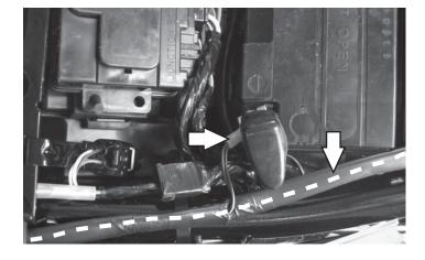
Attach the ground wire from the PC6 harness to the negative side of the battery.
