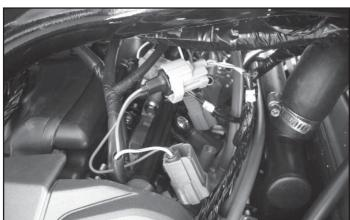
11 Locate the primary throttle position sensor on the right hand side of the throttle bodies.
