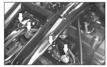
10 Attach the connectors from the PC6 to the stock wiring harness and injectors.
