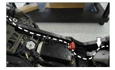
5 Continue routing the wiring harness under the fuel tank and towards the throttle bodies following along inside the left side frame spar.
