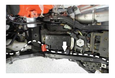
4 Lay the PC6 module in the tail section and route the wiring harness along side the stock wiring harness towards the engine.
