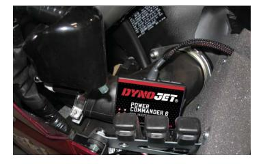
Using the supplied Velcro, secure the PC6 to the left hand ram air tube as shown.
