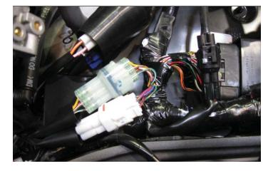
5 Unplug the wiring harness from the throttle bodies.
