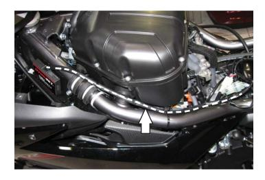
4 Route the PC6 harness down the left side of the air box and go towards the throttle bodies.
