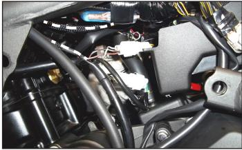
12 Plug the PC6 wiring harness in-line of the stock CPS connectors.
