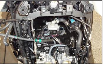
14 Plug the PC6 wiring harness in-line of both Ignition Coils and the stock wiring harness (Fig. L).
