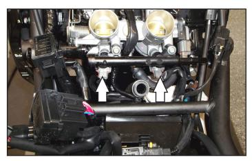
10 Plug the PC6 wiring harness in-line of both Fuel Injectors and the stock wiring harness.
