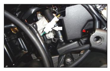
11 Locate and unplug the stock Crank Position Sensor connectors.
