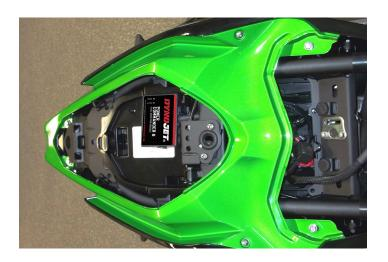
Secure the PC6 module in the tail section beneath the passenger seat.
