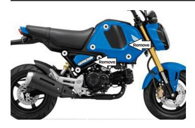
Remove the seat, and side panels from both sides.
