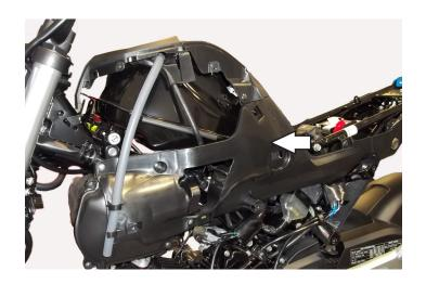
2 Remove the inner panel from each side of the fuel tank.
