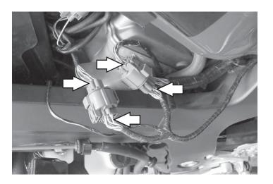
4 Plug the GREY connectors from the PC6 in-line of the stock connectors.
