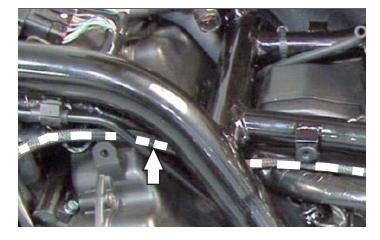
5 Route the PC6 wiring harness forward towards the engine following alongside the stock wiring harness beneath the left side frame rail.
