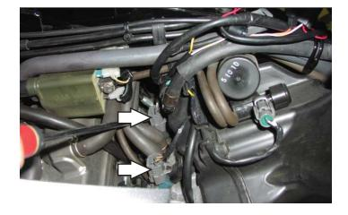
5 Unplug the stock wiring harness at injectors #1 and #2.
