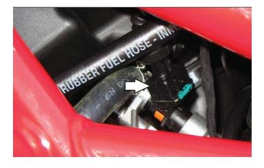
4 Unplug the stock wiring harness from the rear fuel injector.
