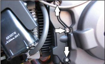
11 Remove the BLACK plastic engine cover on the left side of the bike by removing the three bolts.
