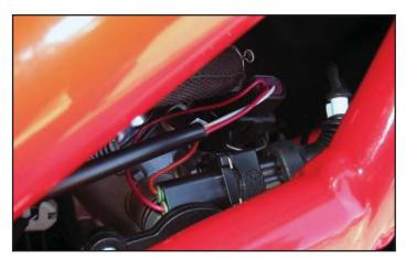
8 Locate and unplug the stock Throttle Position Sensor (TPS).
