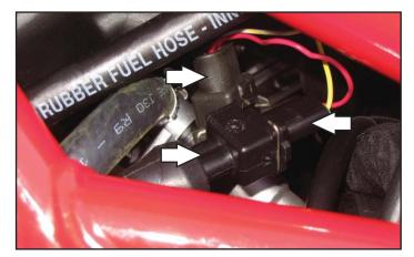
6 Unplug the stock wiring harness from the front fuel injector.
