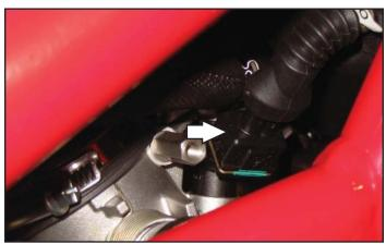
7 Plug the pair of PC6 leads with the ORANGE colored wires in-line of the front fuel injector and the stock wiring harness.
