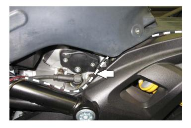
3 Continue routing the PC6 harness along left hand side of the frame.
