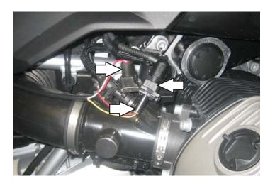
4 Plug the pair of leads with yellow colored wires from the PC6 in-line of the right side fuel injector and the stock wiring harness.
