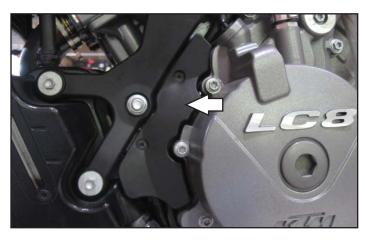
13 Remove the small plastic cover on the left side of the engine.
