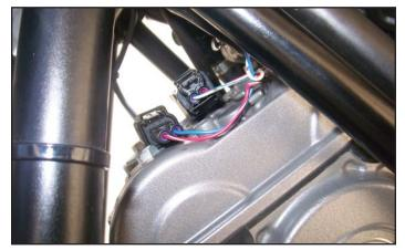
8 Locate the stock connector from the throttle bodies on the right side of the motorcycle. Unplug this connector.
