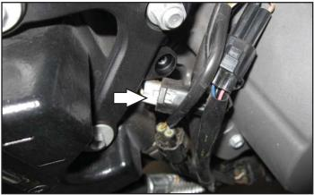
14 Unplug the stock Crank Position Sensor connectors.
