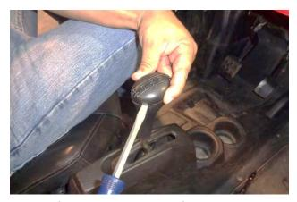
2. Carefully remove the stock shifter handle cap with a flat tip screwdriver or plastic trim tool.
