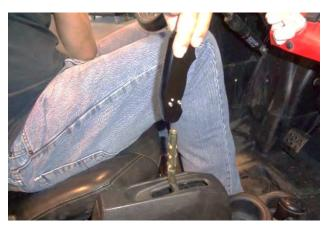
Slide the shifter handle body all the way onto the shifter lever.
