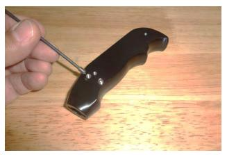
4. Thread the 4 set screws (Item 5) about 2-3 turns into the shifter handle body (1). (Two screws each side.)
