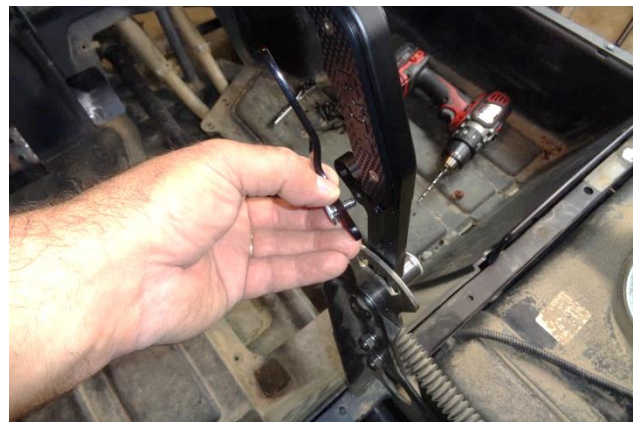
19. Remove the locking lever from the shift lever assembly. NOTE: Do not lose the small spring washer that is under the bolt head.
