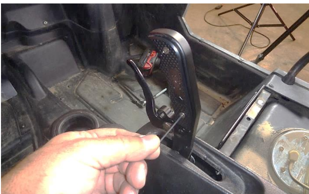
23. Reinstall the two side plates.
