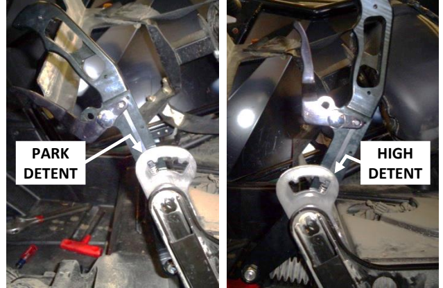
17. Move the shift handle from PARK to HIGH and back several times, releasing the locking lever at both positions. If the selector pin falls into both the PARK and HIGH detents when the locking lever is released, the shift cable is correctly adjusted.
