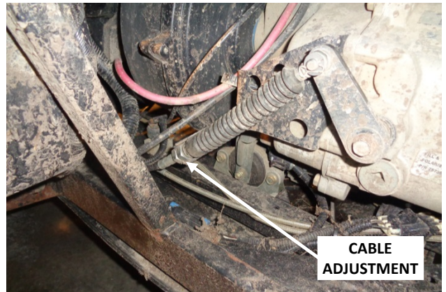
18. If the selector pin only falls into one of the detents, adjust the shift cable according to your owner or maintenance manual.
