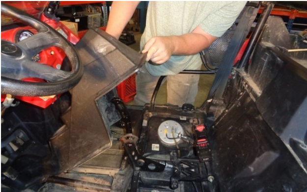
21. Install the center console.
