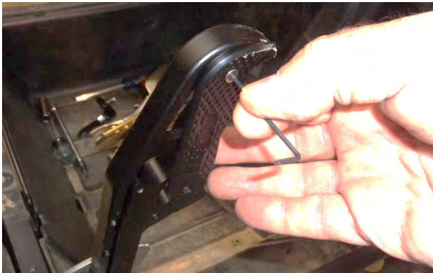
20. Remove both side plates.
