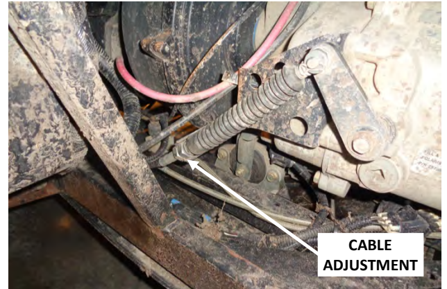
18. If the selector pin only falls into one of the detents, adjust the shift cable according to your owner or maintenance manual.
