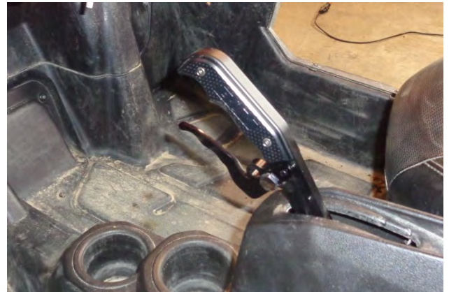
25. Reinstall the seats in the vehicle. Congratulations, the installation of your XDR Off-Road Magnum Grip Hill Killer Gated Shifter is now complete!
