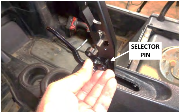
22. Reinstall the locking lever, spring washer and bolt. Ensure that the lever properly engages the selector pin.
