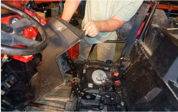
21. Install the center console.
