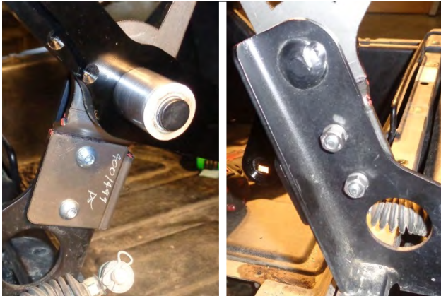
15. Fasten the gate to the shifter support frame using the screws (2) (on the passenger side), and lock washers (4) and nuts (5) (on the driver side).
