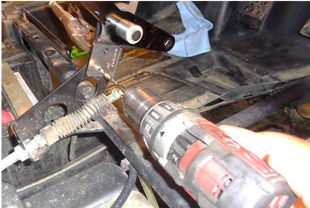
14. Using the holes in the gate as guides, drill two 1/4" holes through the shifter support frame.
