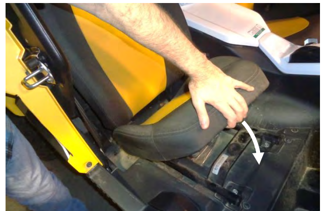
41. Reinstall the seat cushion. First slip its rear tabs under the retaining rod, then push the cushion down firmly until its pin snaps into the grommet.
