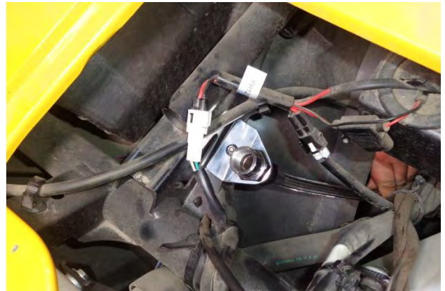
27. Fasten the dipstick bracket to the vehicle frame using the M6 screw (6) (on the bracket side), and the flat washer (7), lock washer (8) and nut (9) (on the frame side).
