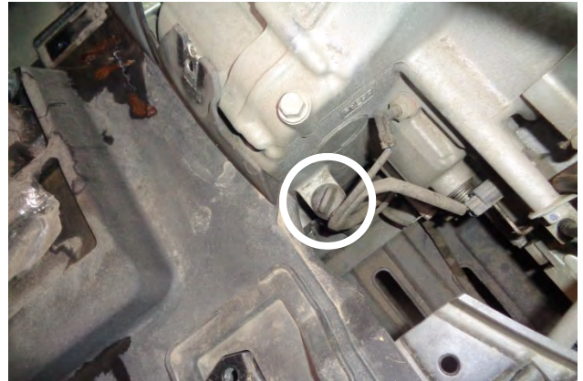
11. Clean the filler cap and surrounding area to prevent loose dirt from falling into the fill port. Then remove the cap, wipe the dipstick with a clean rag, and insert it back into the case without screwing it in (let it just rest on the opening).
