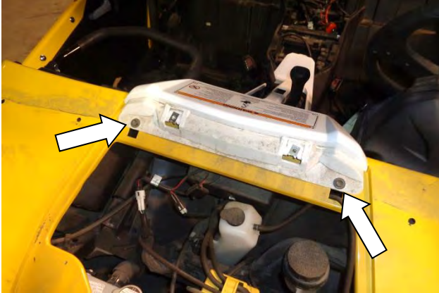
7. Remove the two screws at the front of the front console cover.
