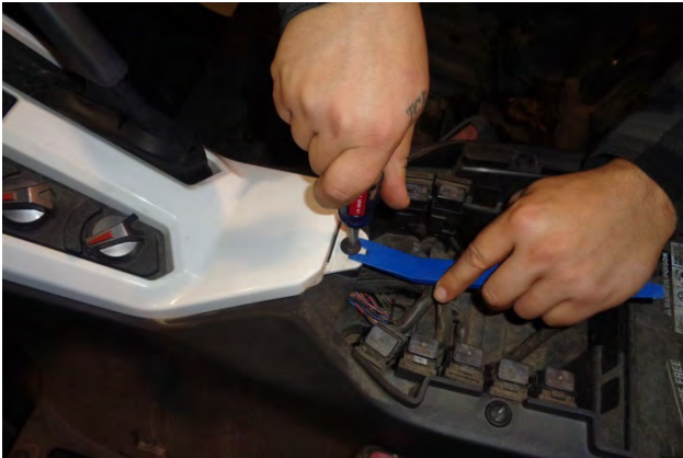
8. Use a plastic trim removal tool and a screwdriver to remove the plastic push rivet at the rear of the front console cover. Then remove the cover.
