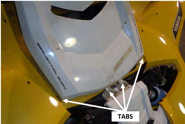
35. Insert the four tabs at the front of the service cover into their respective slots and lay the cover in place.
