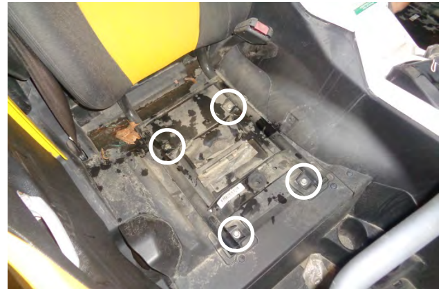
38. Reinstall the seat back, fastening it to the vehicle with its four bolts.
