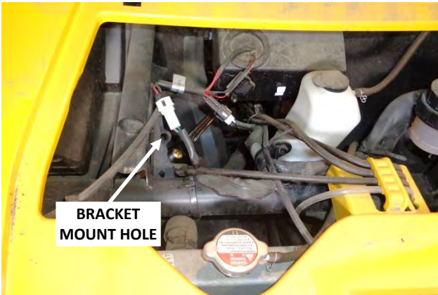
24. In the service compartment, locate the frame hole to which the dipstick bracket will be attached, and route the tube toward the hole.
