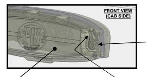
As shown on the front-view image, the <u>lever</u> is installed by default on the right side of the vent.
