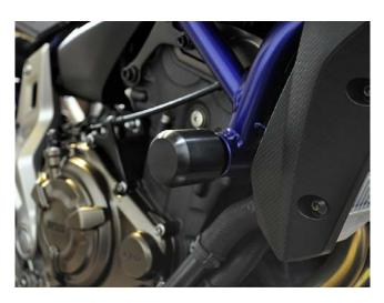
3) Slide the plastic slider over the top of the base and secure it in place using the 8 mm countersunk bolt provided. The bolt passes first through the non threaded hole and then screws into the threaded hole on the far side of the base. The plastic is undersized on the far side of the slider to act as a locknut for the bolt.
