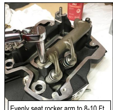
Evenly seat rocker arm to 8-10 Ft. Lbs, loosen to allow shaft to settle then evenly step torque to final 24-26 Ft. Lbs. Verify rocker
