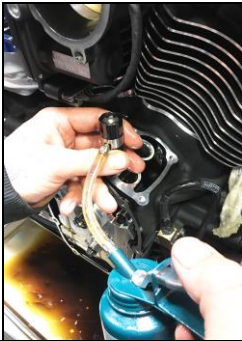
Manually pump up lifters
