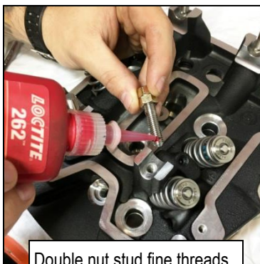
Double nut stud fine threads & Loctite course threads
