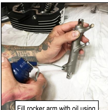
Fill rocker arm with oil using a oil squirt can
