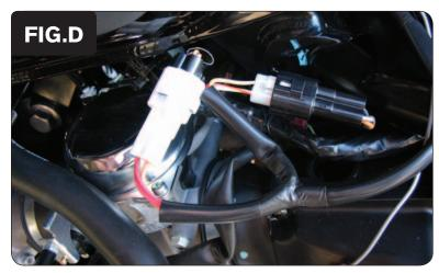
8 Plug the PCV harness in-line of the stock connectors (Fig. D)
