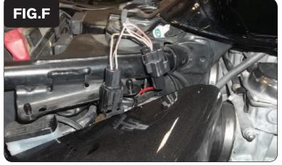
10 Plug the PCV in-line of the stock Crank Position Sensor connectors (Fig. F).
