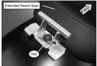
3. Remove the rear fender screw and washer. Install Extended Reach Passenger Seat (A01) by engaging the front seat base tabs onto the bracket (A02), then lower the back of the seat to the fender and install the rear screw and washer. Tighten the screw to 17 Nm (12.5 ft lb). Ensure that the front seat tabs fully engage the bracket (A02).
