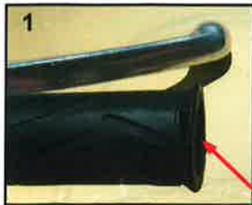
Bar Weight Removed
