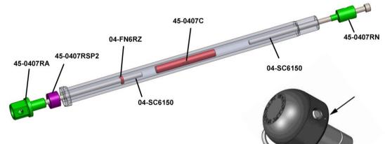
**Important:** One side of the puck has a small hole drilled beneath the main hole. Install the pin so that the end of the pin with the ball is on the same side as this small hole. The pin should be installed so that the ring is on the upper half of the slider.
