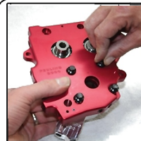
Bolt oil pump to camplate finger tight DO NOT use loctite or hardening compound
