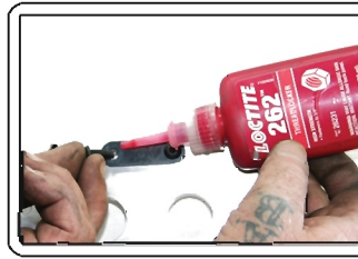
Apply Loctite to block off plate bolts
