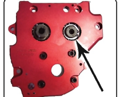
Install retaining ring
