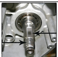
Remove burrs & scoring from pinion shaft to assure smoothness
