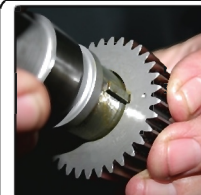
Line up gear with camshaft
