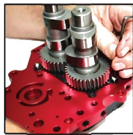
Install bearing retainer plate using loctite
