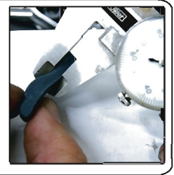
clay pistons and measure thickness of clay after cycling engine
