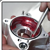
Apply engine assembly lube to oil pump housings & gears
