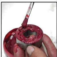
Apply engine assembly lube to oil pump housings & gears
