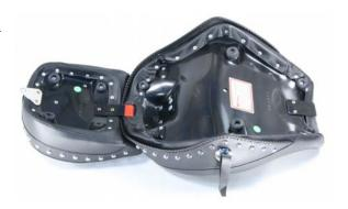
2. Lift the stock seat up and back to remove from motorcycle.
