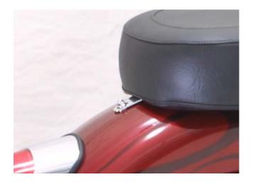
5. The bracket will be up to 1" above the rear mount. Push down on the rear of the seat, flexing the fiberglass baseplate, ensure all bumpers are directly contacting the fender, and secure with the stock acorn nut.
