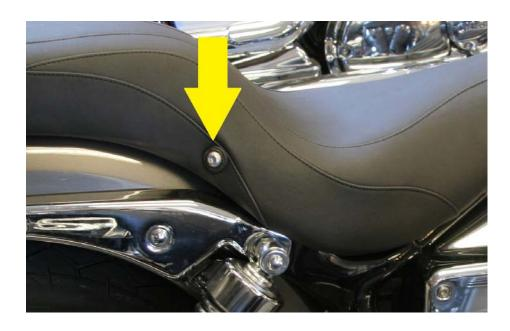
2. Insert the two stock rubber bushings through the sides of the seat. A small X has been pre-cut in the vinyl. Check to be sure the bushings line up to the seat's brackets and the frame mounting points.
