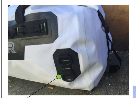
Anchor patches are plates of high-strength 1680d fabric which have handles, D-rings and daisy chains sewn to them. The patches are then welded to the bag body providing a bomb proof solution not found on most dry bags but needed for high stress scenarios of motorcycle use.
