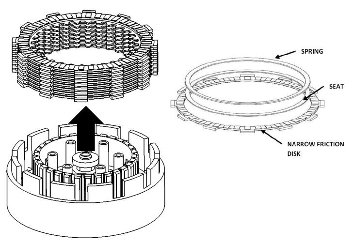
6. Inspect the basket for cushion slop or notching. If notched or worn, it is recommended to replace the basket. See Read Me First for more inspection information. **Do not install sleeves or use product with a notched basket.**
