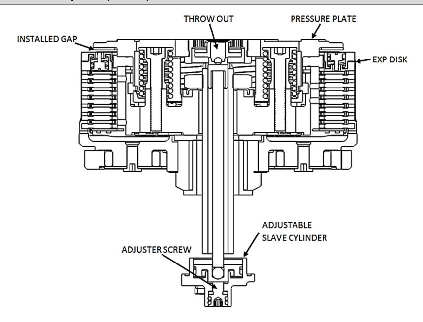
25. Using the long end of a 4mm Allen key, turn the adjuster screw clockwise until it stops under moderate pressure. You are trying to feel for the point at which the throwout will start to lift the pressure plate. This is the "starting point".
