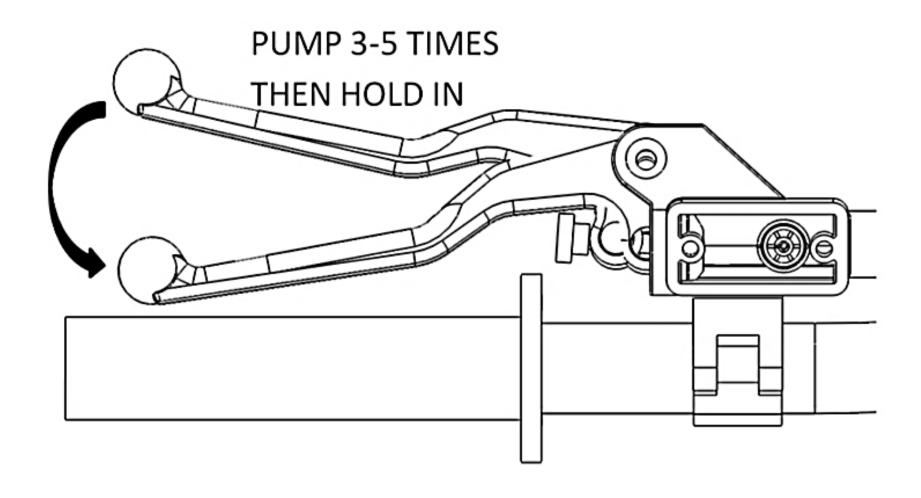
21. Using an 8mm wrench, open the bleed port. Air and fluid should come out of the bleed tube. Tighten the bleed port.
