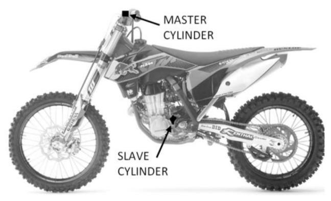
13. Starting at the slave cylinder, remove the OEM parts named in the following diagram beginning with the banjo bolt.
