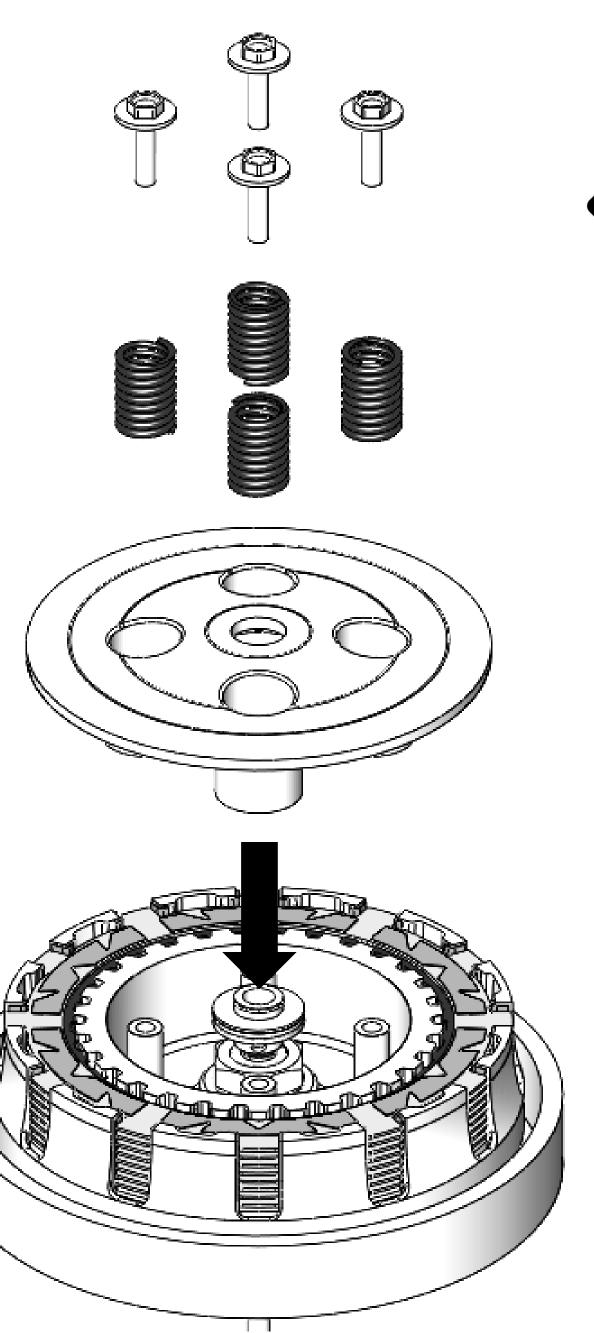
11. Reinstall your OEM clutch cover. Torque Bolts to OEM specification.
