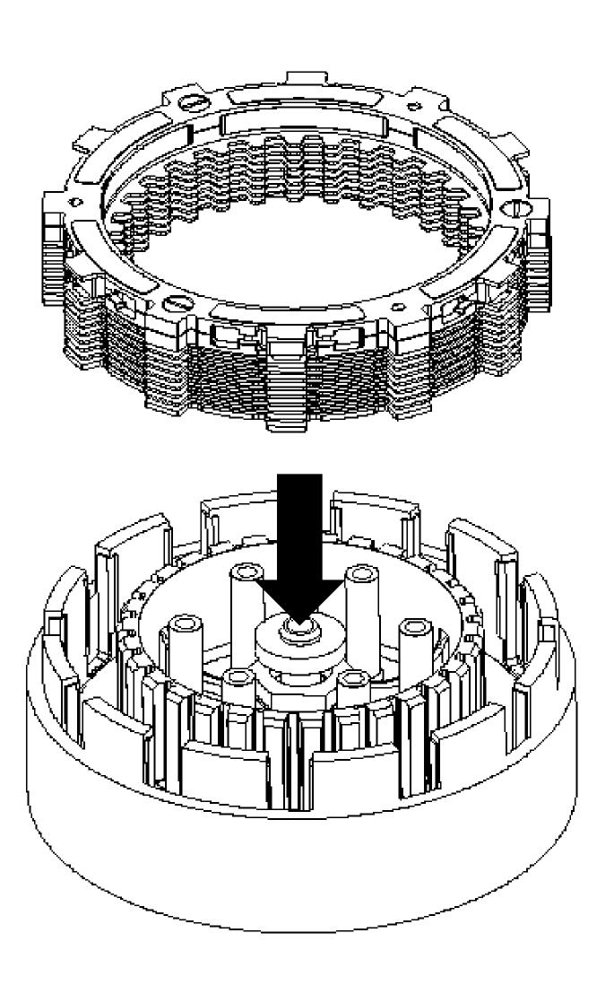
10. Reinstall your OEM pressure plate followed by the provided the Rekluse pressure plate springs, and the OEM pressure plate bolts. Torque bolts to OEM specification.
