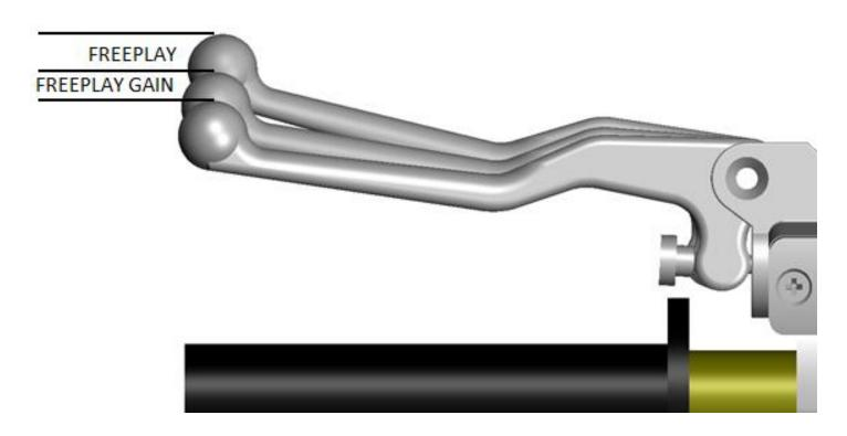
Optimal Free Play Gain yields 1/8-1/4" (3mm-6mm) of clutch lever movement, measured at the end of the lever. This measurement at the lever correlates to achieving the ideal installed gap.
