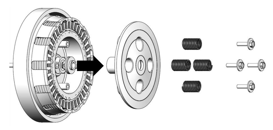
5. Remove and set aside the OEM clutch pack. (All Plates)
