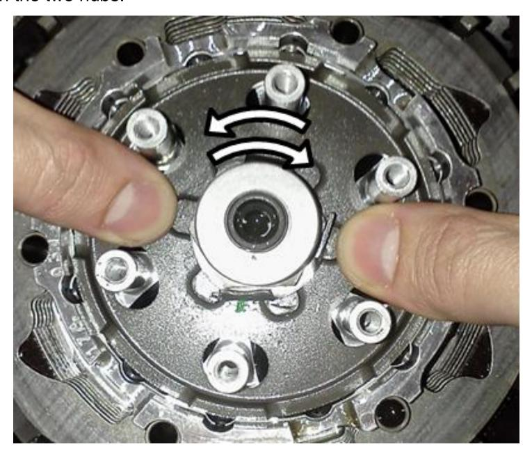
6. Install the Rekluse clutch pack as seen in the configuration on the following page.
