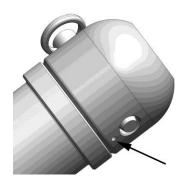
3) Install the plastic top using the removable pin. **Important**: One side of the puck has a small hole drilled beneath the main hole (see picture at left). Install the pin so that the end of the pin with the ball is on the same side as this small hole. The pin should be installed so that the ring is on the top half of the slider.
