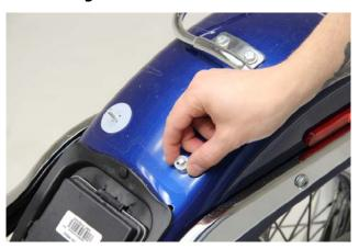
1. Remove one of the large retaining washers from the fender studs and replace with the supplied small retaining washer. Repeat for other stud.
