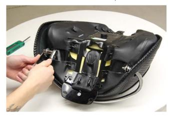
4. Using two 3/8" hex wrenches, loosen the nuts holding the sides of the chrome rail to the stock solo. Using a T30 Torx wrench, remove the central rear bolt which connects the solo's rear bracket to the chrome rail. Carefully disengage the chrome rail from the stock solo.
