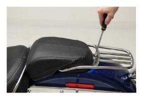
2. Remove the threaded spacer and washer from the rear mount hole on the rack using a ½" hex wrench. (This spacer will not be used to mount the Mustang passenger seat.)
