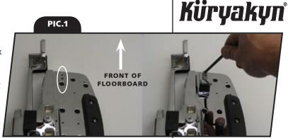
**STEP 4** Using a 6mm hex key or driver, remove the two socket screws that hold your shift side OEM peg mount to the frame and remove the OEM peg mount. See <u>PIC.2</u>. Set the OEM hardware aside, it will be reused.
