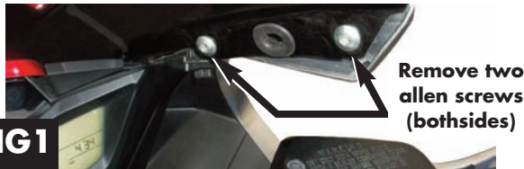
Fig 1. Remove both mirrors. Locate both fasteners located on the inside fairing. Also, remove inner plastic that's covering both left & right two allen screws.
