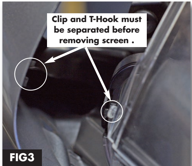
Fig 3. Separate T-Hooks from the retention clip by applying a light pressure from the corner fairing and work the light pressure down as shown. (Both Sides) Be careful not too exert to much force!
