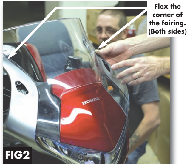
Fig 2. After removing the mirrors, flex the corner fairing to expose the next step in unhooking the stock windscreen as shown in Fig 3 .
