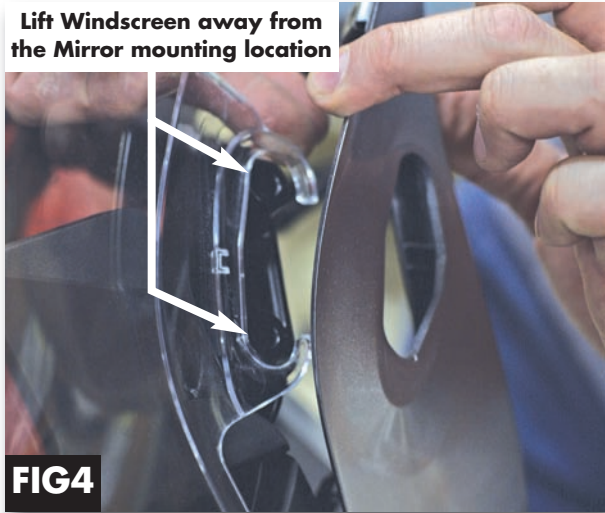
FIG 4. Locate the upper fairing, Lift windscreen away from the mirror mounting standoffs. It should look like this on both sides of the windscreen.
