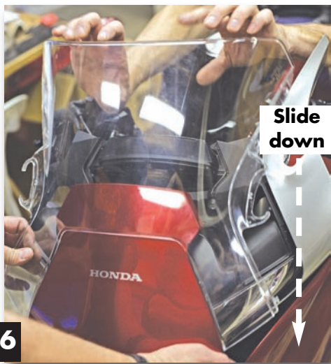
FIG 6. Now you are ready to unlock the screen from the fairing. Apply light pressure from the top of the back side of the finish plate . There are three retention locations on top to dislodge and also one located at the very bottom of the finish plate. Apply light pressure separating the clip from the fairing, and slide the windscreen/finish plate down. Note: The finish plate is attached to the stock windscreen.
