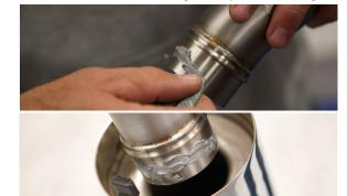
3. Loosely slide supplied barrel clamp on TBR slip tube.
