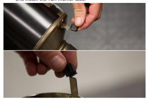
Be sure to remove OEM joint gasket. This will NOT be re-used.
