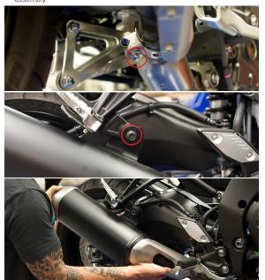
3. Remove OEM muffler mount bracket from right passenger peg.
