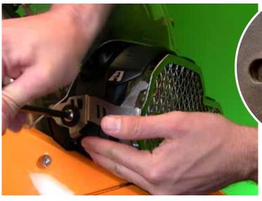
Peaking in behind the stainless arms, you can make sure your aiming marks are lined up properly. Pushing on the headlight guard from the front, make sure the support tab contacts the headlight frame. This ensure the headlight guard holds its position even in the toughest conditions.
