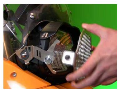
6 Install the front face of the Headlight Guard. Line up the holes in the face, with the 1/4-turn fasteners, then turn the fasteners to engage the mechanism.
