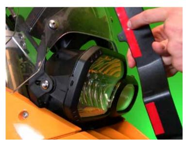
Now remove the backing on the adhesive tape. \*Ideal application temp range is 70 to 100 F. Min suggested application temp is 50F.
