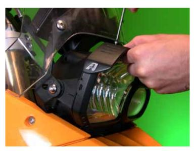
Have the T-15 Torx fastener in the mounting hole, and use it to align the Glare Guard on the top of the bezel. Once the fastener is tightened, press firmly on the bezel to ensure the adhesive bonds well.
