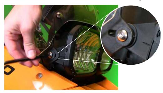
Using a T-30 torx tool, loosen both the left and right fasteners that hold the Headlamp in place. Notice the aiming marks. Also remove the T-10 Torx screw on the top of the bezel.
