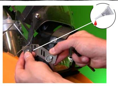
Line up the arm using the tabs to interface with the headlight frame. for each side and insert the OEM fasteners with one drop of thread locker on the last couple of threads and turn just a few turns.
