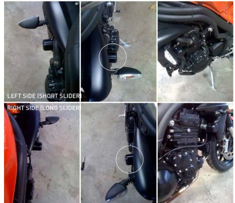
3) Slide the plastic slider over the top of the base and secure in place using the 6 or 8 mm countersunk bolt provided. The bolt passes first through the non threaded hole and then screws into the threaded hole on the far side of the base. The plastic is undersized on the far side of the slider to act as a locknut for the bolt
